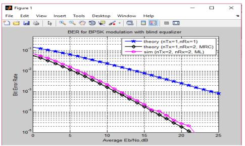
Fig 7. BER for BPSK modulation with blind equalizer
