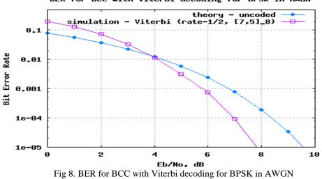
BER for BCC with Viterbi decoding for BPSK in AHGN
